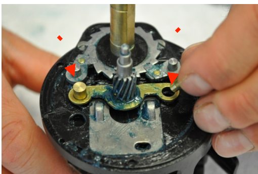
Step 19: Install yoke pins
