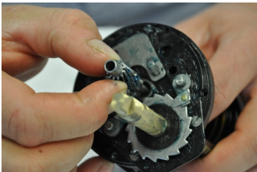
Step 17: Install the new pinion gear on to the main shaft. (note square side of the pinion gear should be facing down towards inside of reel)
