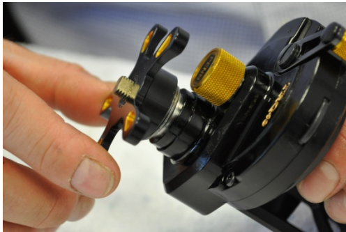
Step 33: Screw the star on by turning clockwise. It will start clicking as it gets tight.
