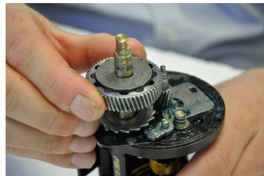
Step 10: Grasp teeth of main gear and slide off the mainshaft. (drag washers located inside main gear will come off at the same time)
