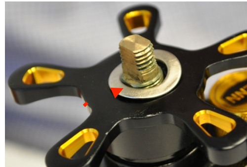
Step 34: Place tension washer on top of star. (note cup/concave side should face down)
