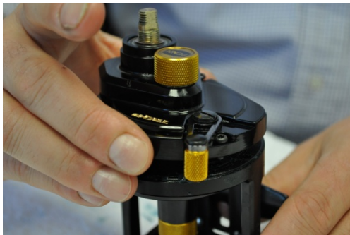
Step 29: Place side plate back on reel. If side plate won't fit flush, check to make sure the anti-reverse dogs are engaged (see step 22)
