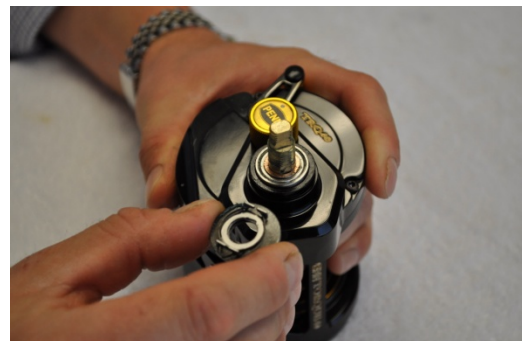
Step 6: Remove detent spring assembly and tension washers located below the star on the mainshaft
