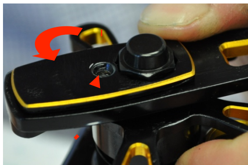
Step 37: Place locking plate over nut and tighten clockwise until the holes lines up for the screw
