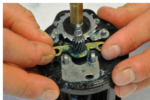
Step 18: Install the yoke. It will fit in the groove between teeth on the pinion gear.
