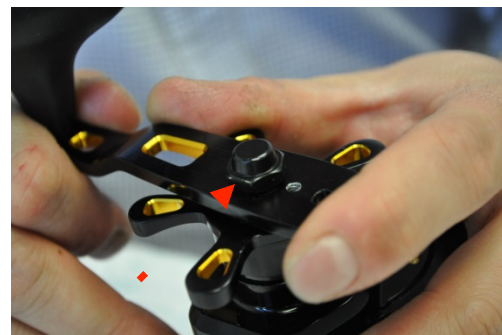
Step 36: Place nut on mainshaft and hand tighten
