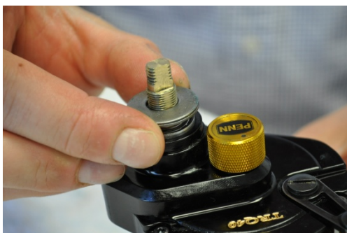
Step 31: Place the two tension washers on mainshaft
