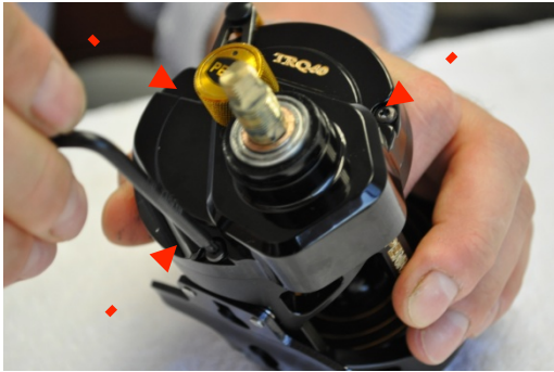
Step 7: Use torx wrench to loosen three screws on side plate
