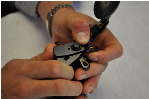
Step 3: Use handle plate to remove the handle nut by turning counter clockwise
