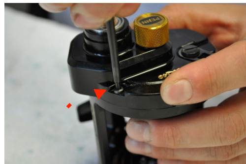
Step 30: Use torx wrench to tighten three screw on the side plate
