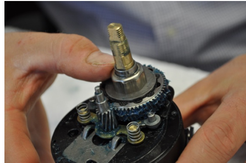
Step 28: Place instant anti-reverse bearing back on mainshaft
