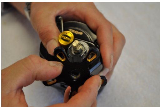
Step 5: Unscrew star counter clockwise and remove from reel
