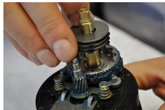
Step 26: Install drag stack on main shaft and place in side the main gear. The slots on the keyed washers will fit inside groves on the main gear.
