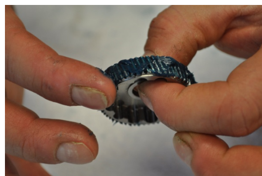
Step 24: Spread grease with fingers or grease brush
