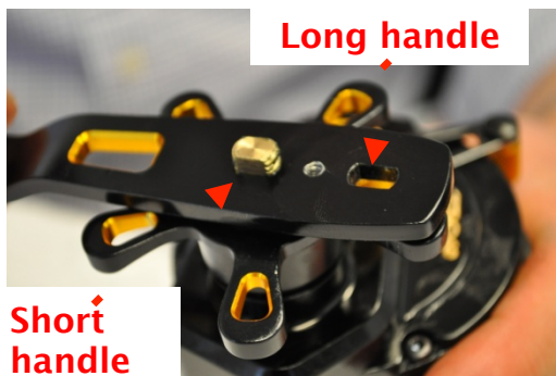
Step 35: Place handle on mainshaft. The length of the handle can be adjusted by placing in the two slots on the handle.
