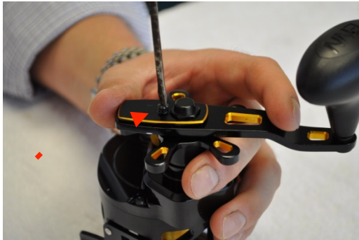
Step 1: Remove handle screw using a small flat head screw driver
