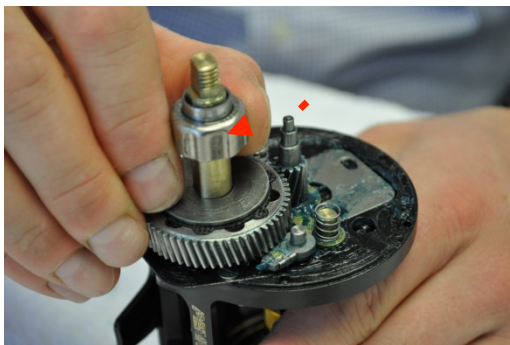
Step 9: Remove instant anti-reverse bearing located on mainshaft
